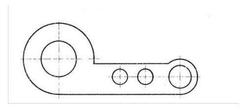
7.Copy the given sketch to 1:1 scale and dimension adopting unidirectional system with combined dimensioning method.
