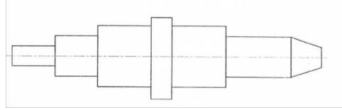
5. Copy the given sketch to 1:1 scale and dimension adopting aligned system with progressive dimensioning method.
