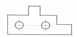
6. Copy the given sketch to 1:1 scale and dimension adopting unidirectional system with chain dimensioning method.
