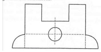
13. Draw the given sketch to 1:2 scale and dimension adopting aligned system with chain dimensioning method
